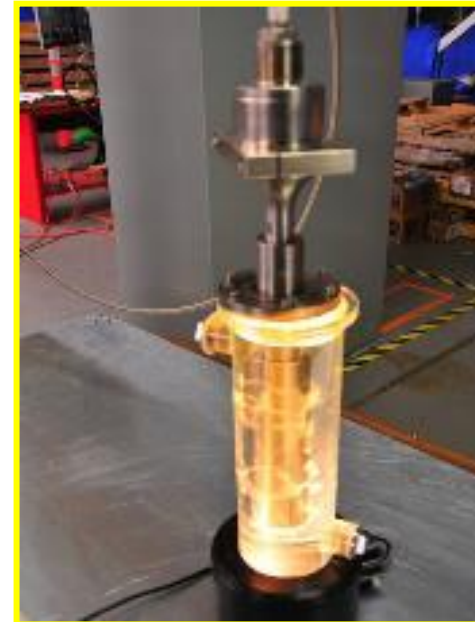
Resonator (reactor) in a flow cell
