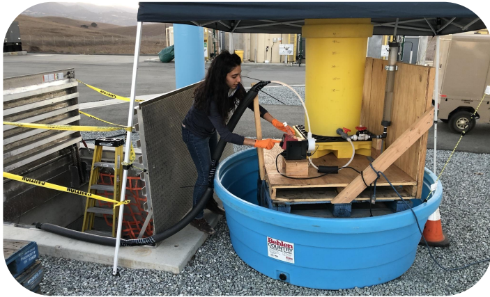
Calibrating Metering Pump
