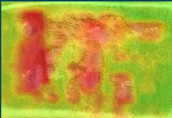
WALL THICKNESS MAP FROM PIPEDIVER ULTRA
