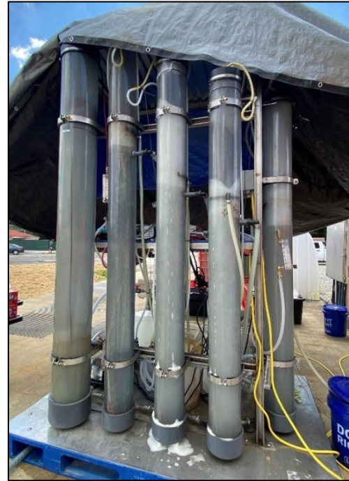
Foam Fractionation (200x PFAS concentration)
