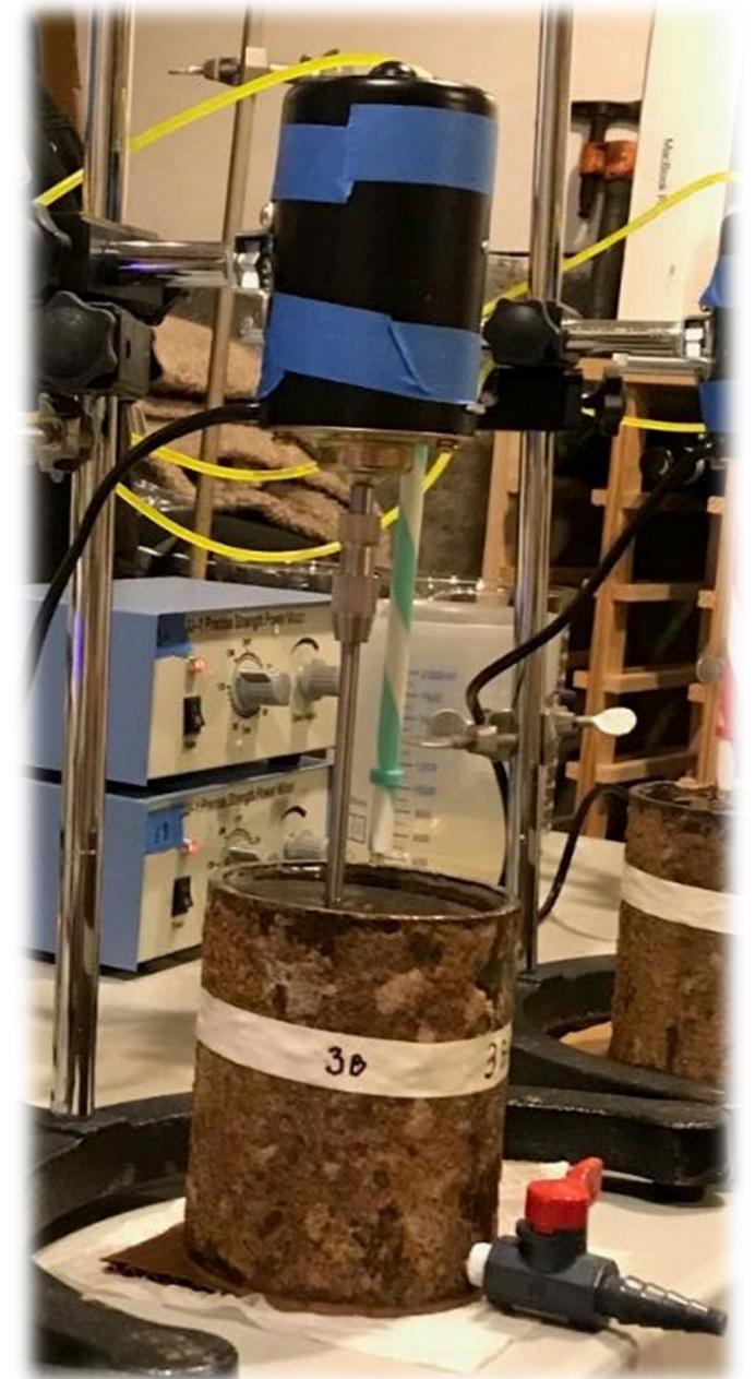
Mixers with small paddles were used for testing
