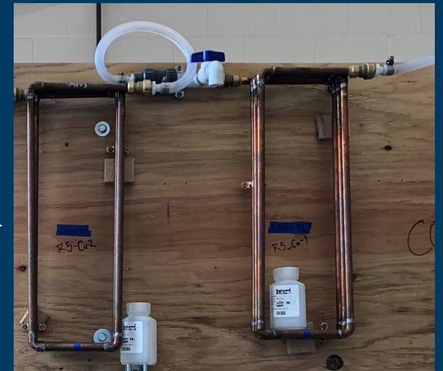
New copper pipe with lead solder
