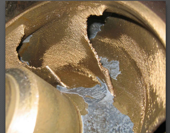
Cavitation damage to an impeller
