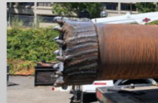
End View of the Cutting Shoe on the 13-5/8-inch Steel Wash-Over Casing
