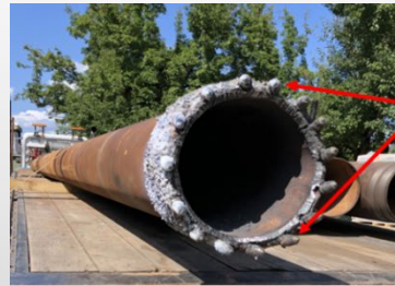
End View of the Cutting Shoe on the 13-5/8-inch Steel Wash-Over Casing
