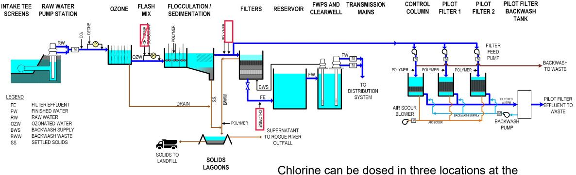
Chlorine can be dosed in three locations at the Duff Water Treatment Facility
