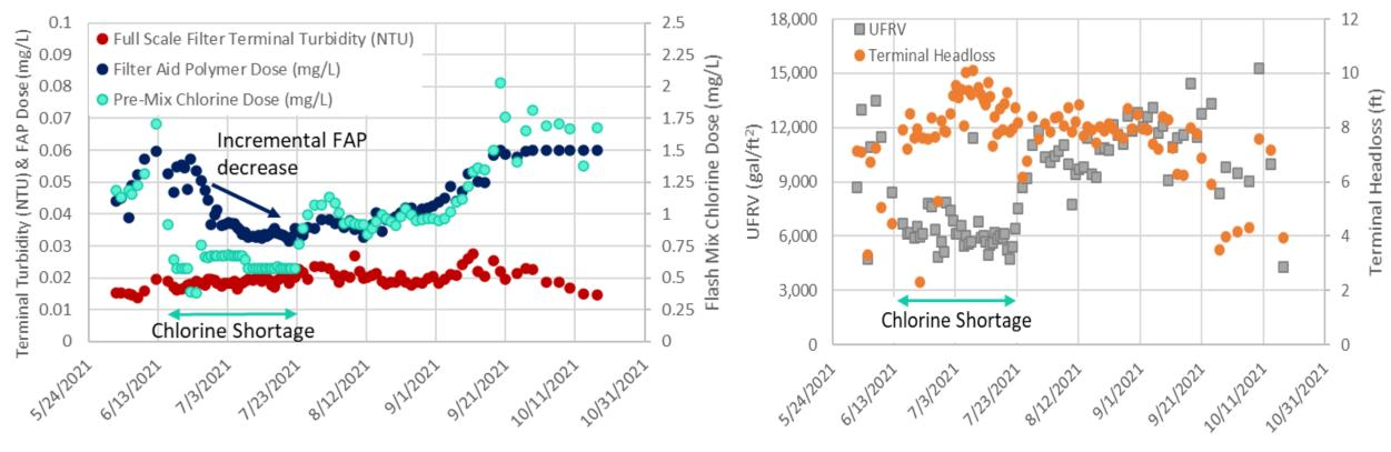
Less pre-oxidation negatively impacted the filter run time and filter aid polymer was decreased in response Full scale filter performance during the sodium hypochlorite shortage
