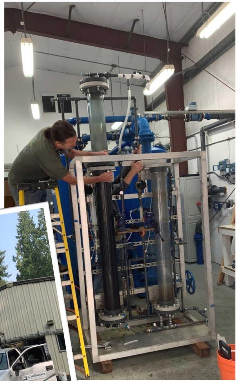
Michael Hallett installing Confluence filter pilot testing equipment
