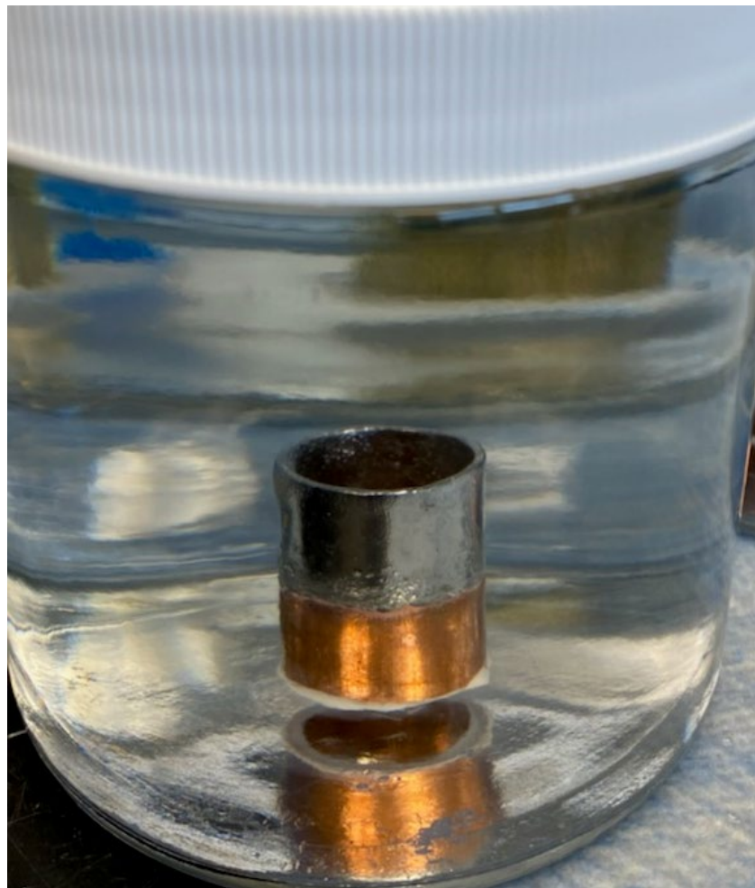
Virgin copper with lead solder coupon
