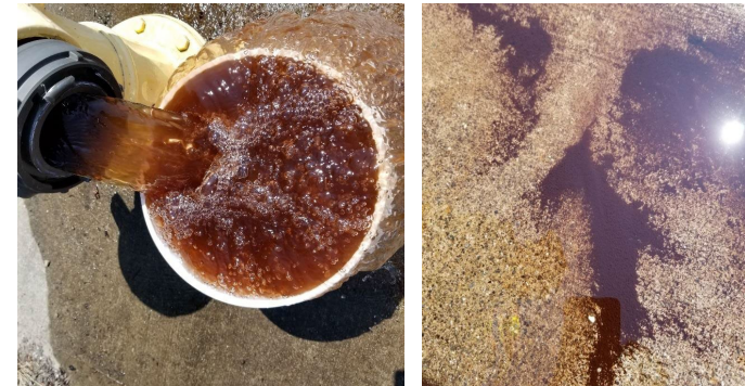
Observed very fine light sediment that is easily stirred up in the main (770 zone) August 2020
