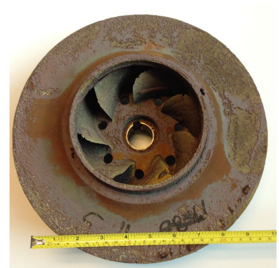
Damaged pump impeller
