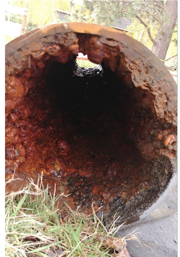
16-inch diameter c. 1926 cast iron (2018)
