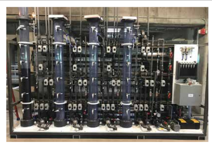
Filter Pilot at JWCD with one column in service.
