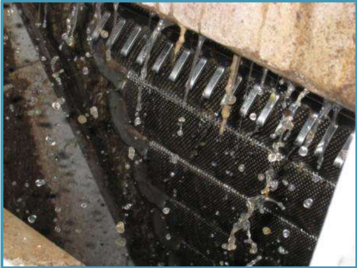
Debris Carryover From Brush and Water Spray
