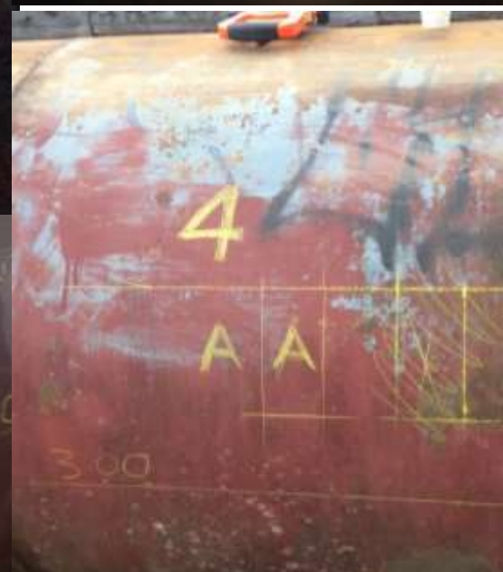
Creating various defects in the calibration pipe
