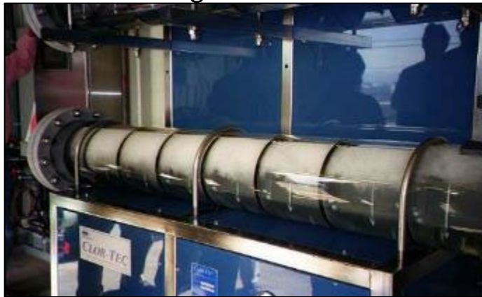
Previous generation utilizes a horizontal cell that is pressurized with a single pass . Note internal hardware, baffles, rupture disks and resultant H 2 blinding of electrodes
