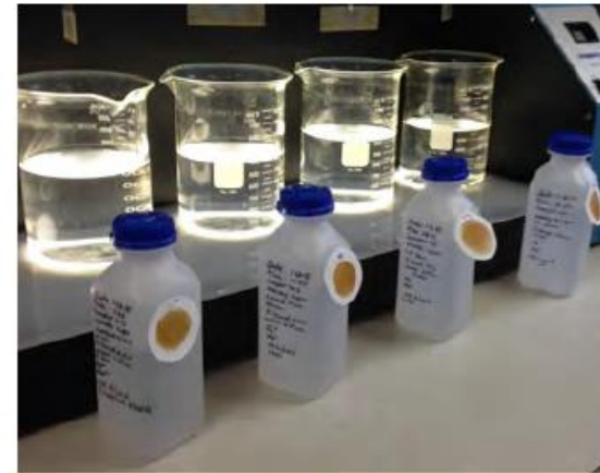
One of our many bench test trials for optimizing the removal of manganese
