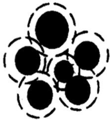
Fisheyes due to poor initial wetting
