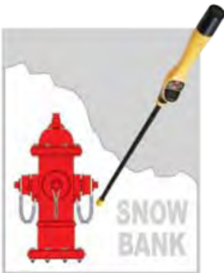
Locator for Buried Hydrants
