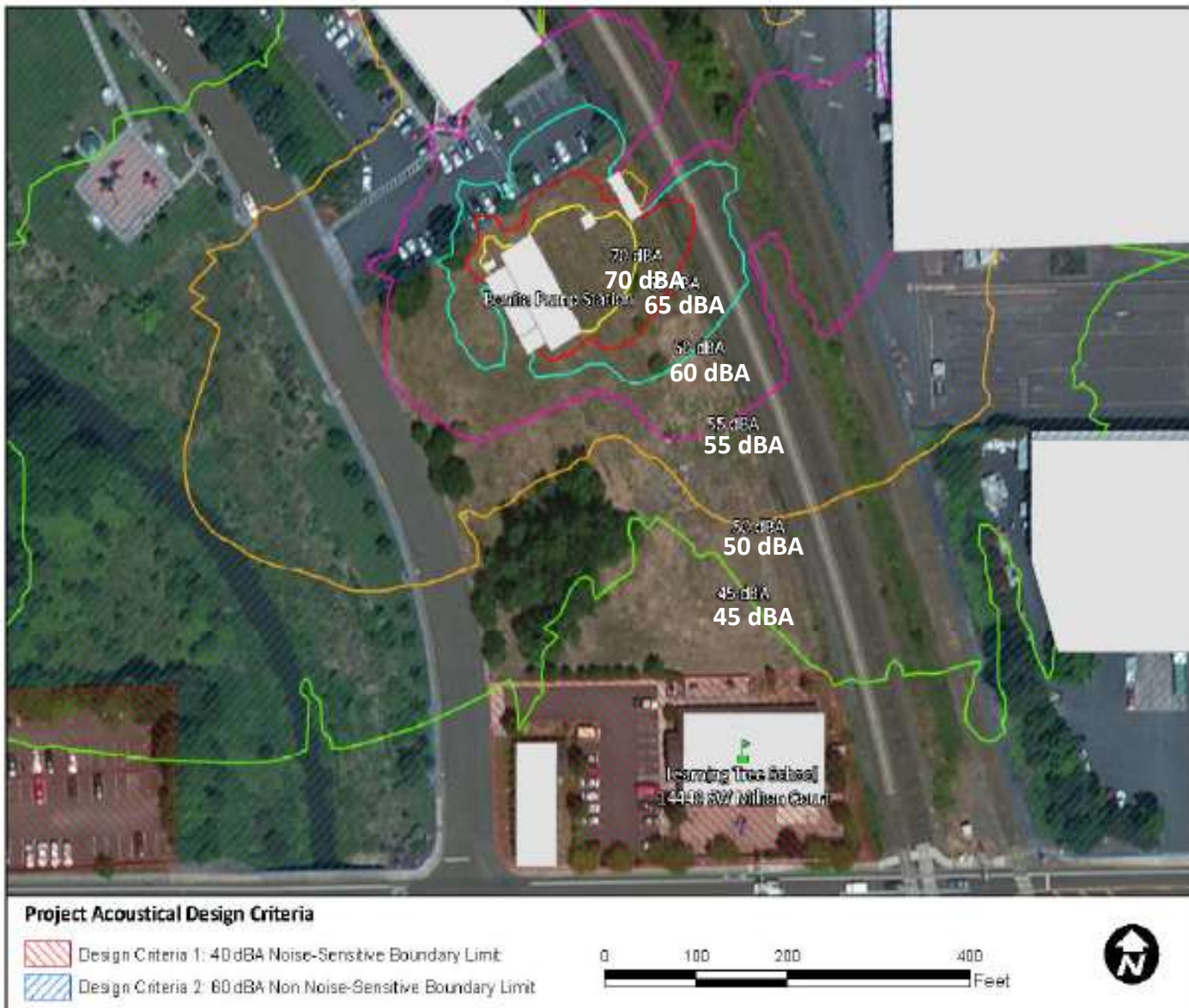
Figure 3-2 Project expected sound levels with standard package equipment (normal operation, excludes engine generator).
