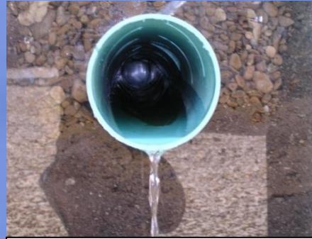
Fixed-Diameter pipes cannot optimize jet velocity
