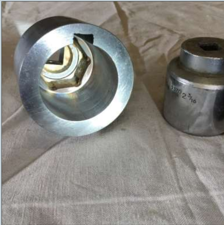
2.5" shaft coupling welded to 1" drive socket.
