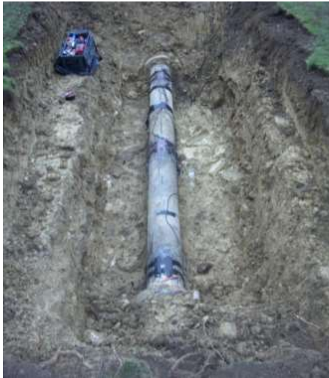
Photos of the one exposed section and the attached Strain Gauges and Temperature Sensors
