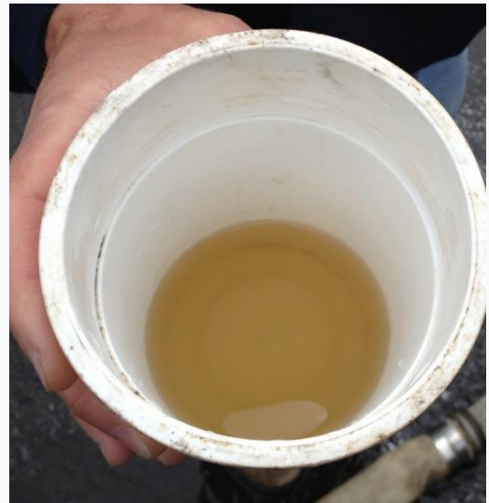
Accumulated particles in Tigard's DS are fine, light, loose, and impart a rust-colored appearance.
