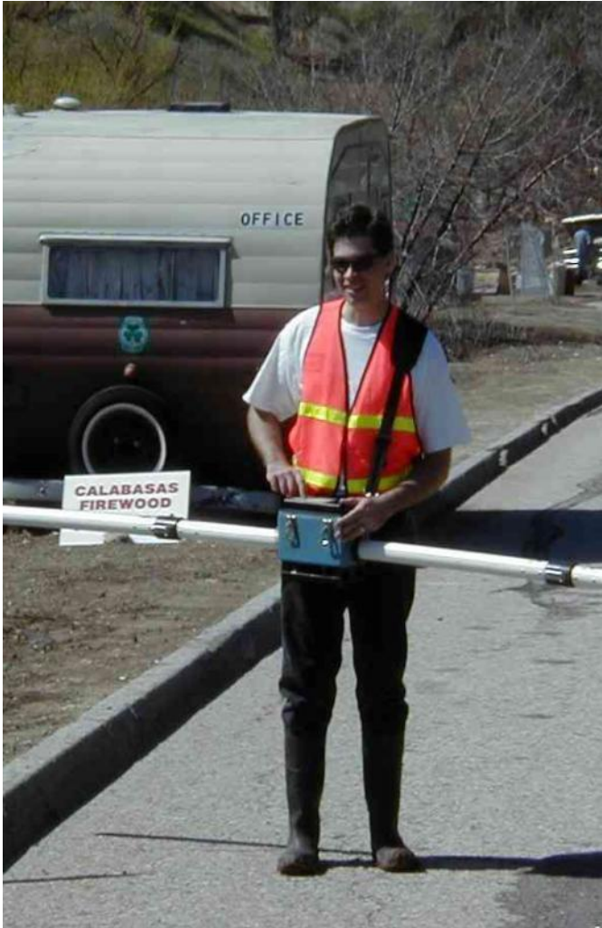
Over-the-Line Corrosion Survey
