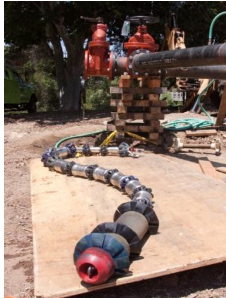
In-Pipe Non-Destructive Exam
