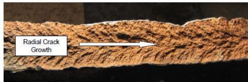
Figure 3-4. Failure morphology along edge of rapid circumferential crack propagation due to beam loading from circular blowout at 12212 Hartsook Street.
