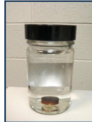
Brass coupon fixed with epoxy to glass bottom
