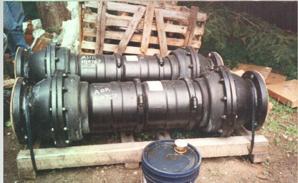
EBBA Flextend connection between tank and yard piping
