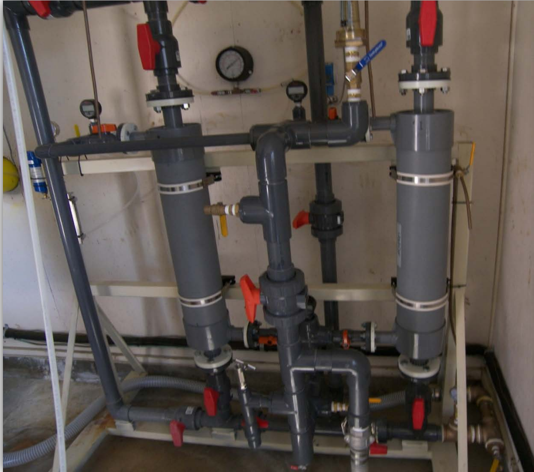
Liqui-Cel 6x28 Pilot Membranes (5-50 gpm) Tested at Well Facility in Sept-2011 and Summer-2010
